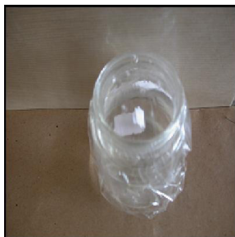
Fig. 5: Tissue wrapped tissue placed in a glass jar containing 99% isopropyl alcohol.
